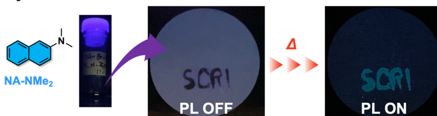
Figure 4. Thermal-responsive behaviors of NA-H/BR-Val-NADI in PL color change for system A and NA-NMe 2 /BR-Val-NADI in PL color change for system B.
