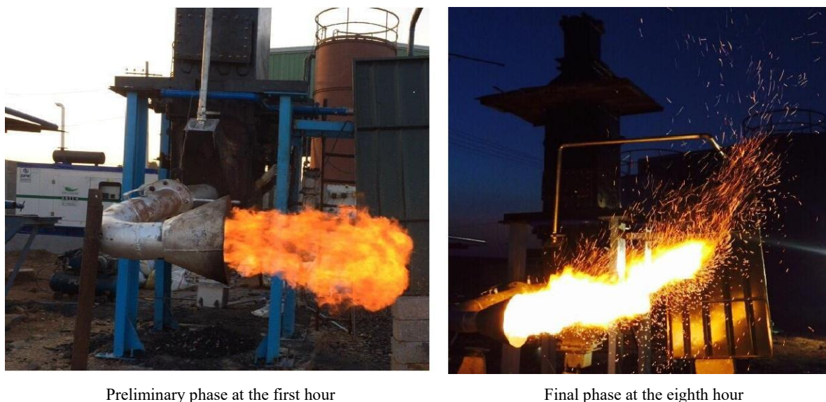
Figure 3. Producer gas flame from MSW gasification utilized at various operational stages.
