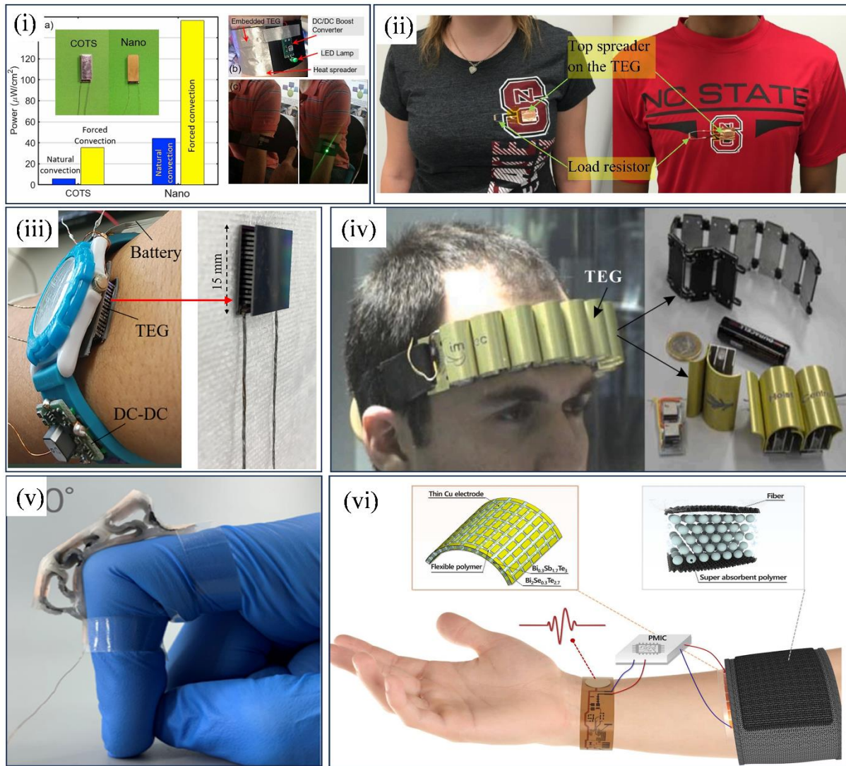
Figure 6. (i) Nanocomposite thermoelectric materials based on Bi 2 Te 3 . “Reprinted with permission from Ref. [48]. 2020, Nozariasbmarz, A.”; (ii) A T-shirt integrated with wearable TEG. “Reprinted with permission from Ref. [49]. 2016, Hyland, M.”; (iii) Wearable TEG supplies power for electronic watches. “Reprinted with permission from Ref. [50]. 2021, Van Toan, N.”; (iv) A brain-computer system powered by wearable TEG. “Reprinted with permission from Ref. [51]. 2008, Van Bavel, M.”; (v) A three-dimensional spring thermoelectric device with basic double elastomer layer and air gap. “Reprinted with permission from Ref. [52]. 2021, Lv, H.”; (vi) A self powered wearable ECG system based on flexible PCB. “Reprinted with permission from Ref. [53]. 2018, Kim, C.S.”
