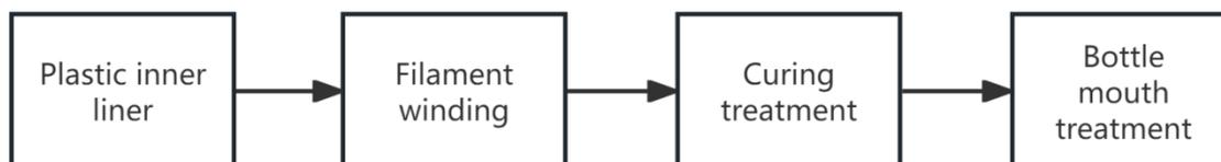
Figure 2. Hydrogen Storage Cylinder Preparation Process.
