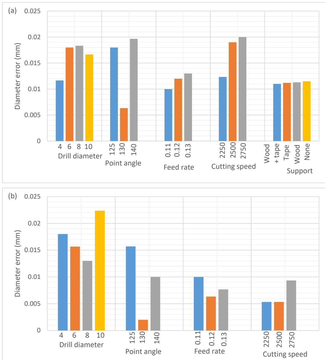
**Figure 7.** Effect of adhesive tape layers on diameter error under varying input parameters: (a) with and (b) without adhesive tape layer.
