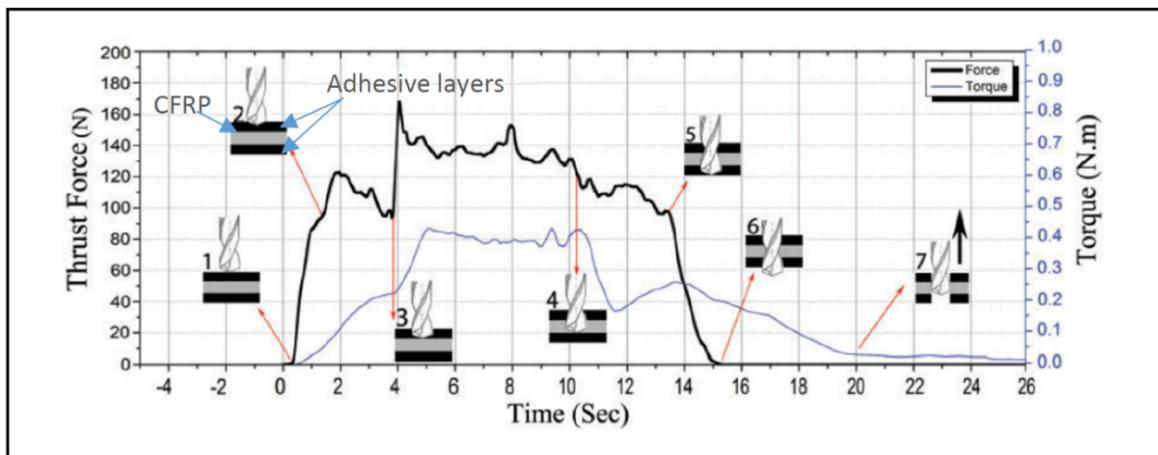
**Figure 9.** Schematic representation of drilling mechanism in terms of thrust force and torque generation with drilling depth.
