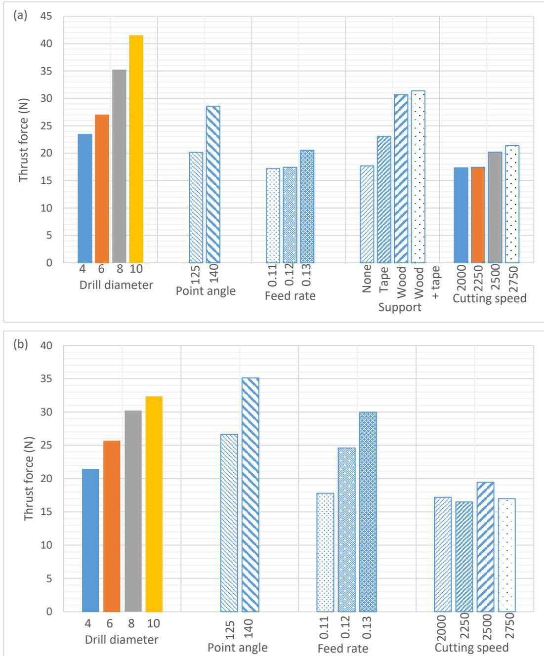
Figure 3. Effect of varying input parameters on thrust force: (a) with and (b) without adhesive tape layer.
