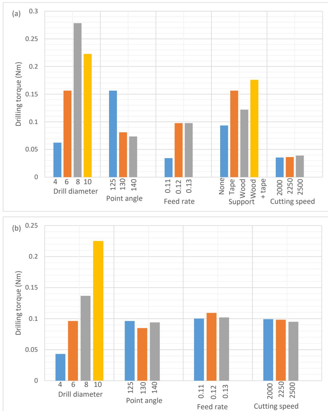
**Figure 4.** Effect of varying input parameters on torque: (a) with and (b) without adhesive tape layer.
