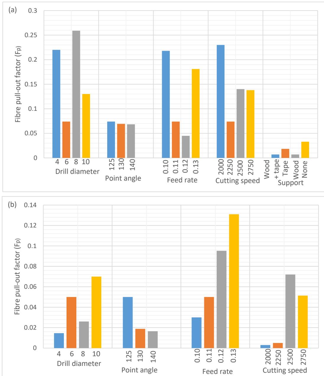
**Figure 6.** Effect of adhesive tape layers on fibre pull-out factor under varying input parameters: (a) with and (b) without adhesive tape layer.
