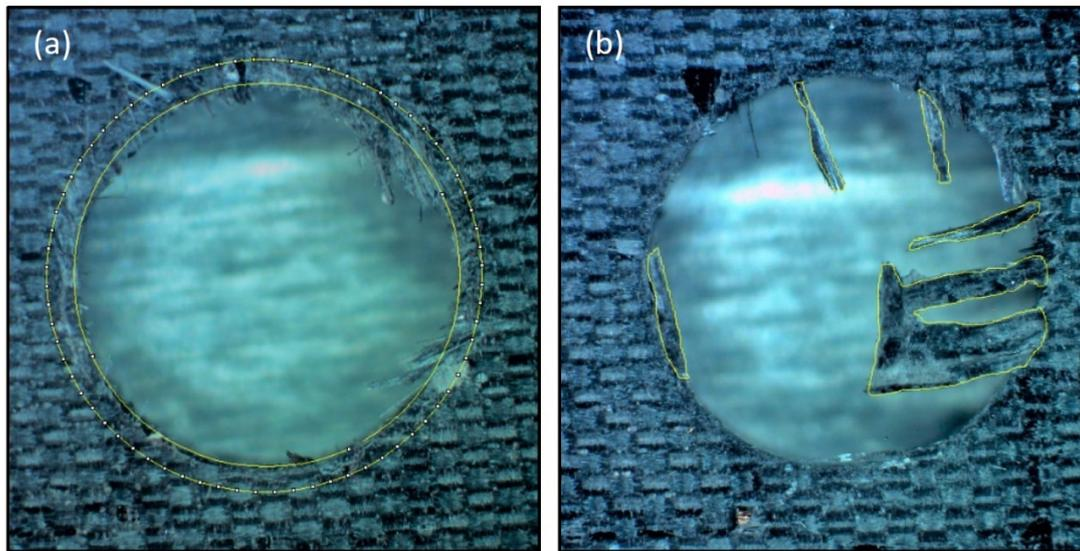
**Figure 1.** Evaluation of (a) delaminated and (b) fibre pull-out zone on holes drilled with following parameters: 0.12 mm/min feed, 2250 rpm with the presence of adhesive tape layers.
