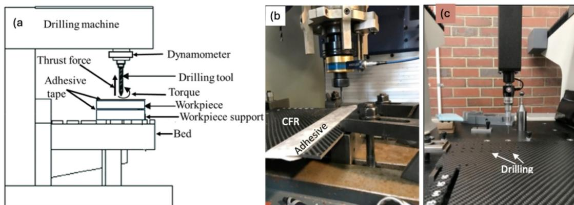
**Figure 2.** (a) Schematic of drilling process, (b) Drilling of CFRP with the presence of adhesive tape layers, and (c) circularity and diameter error measurement with CMM.
