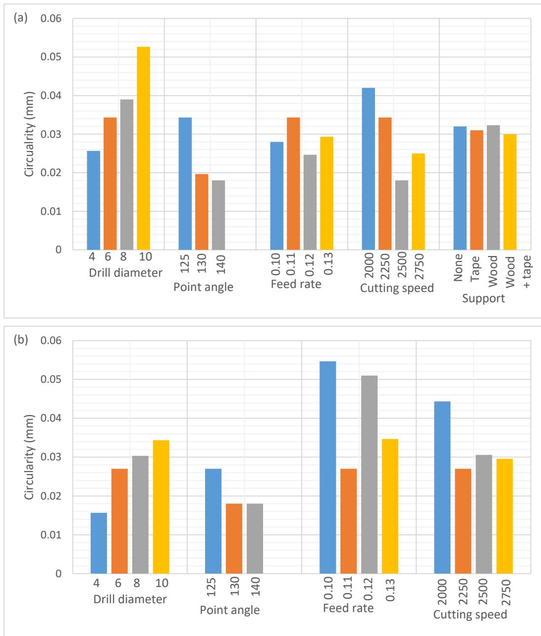
**Figure 8.** Effect of adhesive tape layers on circularity: (a) with and (b) without adhesive tape layer.
