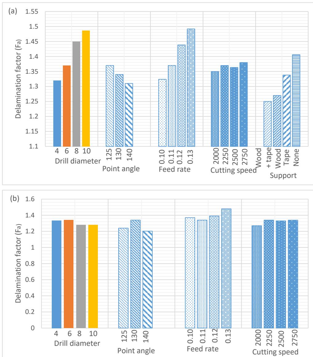
**Figure 5.** Effect of varying input parameters on delamination factor: (a) with and (b) without adhesive tape layer.
