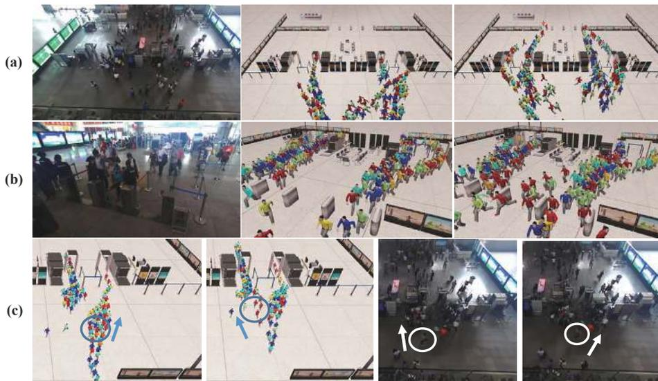
**Figure 16.** The simulation from the real scene: security channels in the train station. (a) The overhead view; (b) The close-up view; (c) The detailed demonstration of dynamic path planning existing in both the simulation and real-world scenario.
