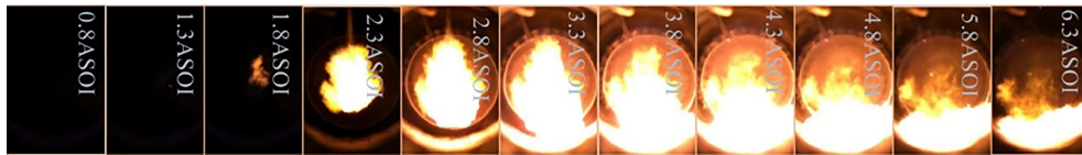
(c) Simultaneous ignition of diesel and methanol.
