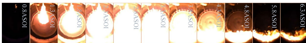
(e) Diesel ignition after methanol combustion.
