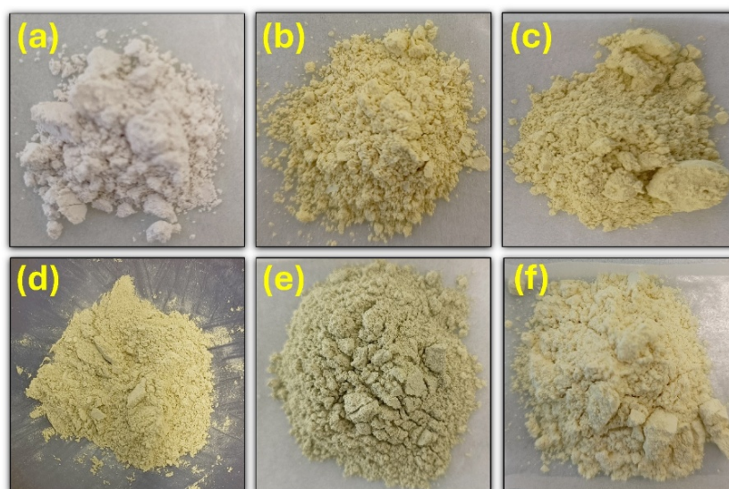
Figure S1. Optical images showing the physical appearance of (a) BTO; (b) 0.5-CN/BTO; (c) 1.5-CN/BTO; (d) 2.5-CN/BTO; (e) 3.0-CN/BTO; and (f) CN.
