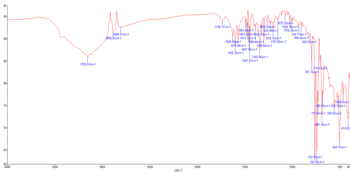
Figure S6. FTIR spectrum of the 2:1 PI:ZrCl 4 system prior to ambient exposure.
