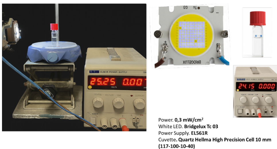
Figure S5. Photograph of the photocatalytic set up used to determine apparent quantum yields in the present study.
