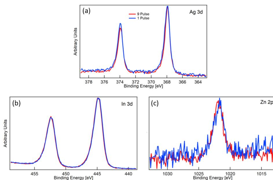
**Figure S13.** Normalized XPS spectra of hybrid TCE made with 9-pulse vs. 1-pulse: (a) Ag 3d, (b) In 3d, and (c) Zn 2p comparing the hybrid TCE made with 9-pulse photonic curing condition (red) and a hybrid TCE made with the 1-pulse photonic curing condition (blue).
