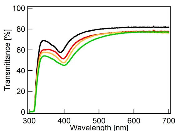
**Figure S14.** UV-Vis transmittance of hybrid TCE and HTL: The UV-Vis transmittance spectra of the hybrid TCE (black) after the sequential deposition of neutral PEDOT:PSS (red), neutral PEDOT:PSS/ PEDOT:PSS (orange), neutral PEDOT:PSS/ PEDOT:PSS/MeO-2PACz (green).
