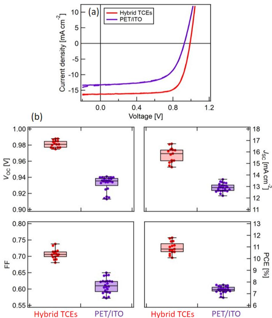
**Figure S15.**  $J$ - $V$  results for hybrid TCE and PET/ITO: (a) Champion  $J$ - $V$  forward and reverse curves and (b) Box plot comparing the average  $J$ - $V$  parameters of the PSCs on hybrid TCEs (Red) and PET/ITO (Purple).
