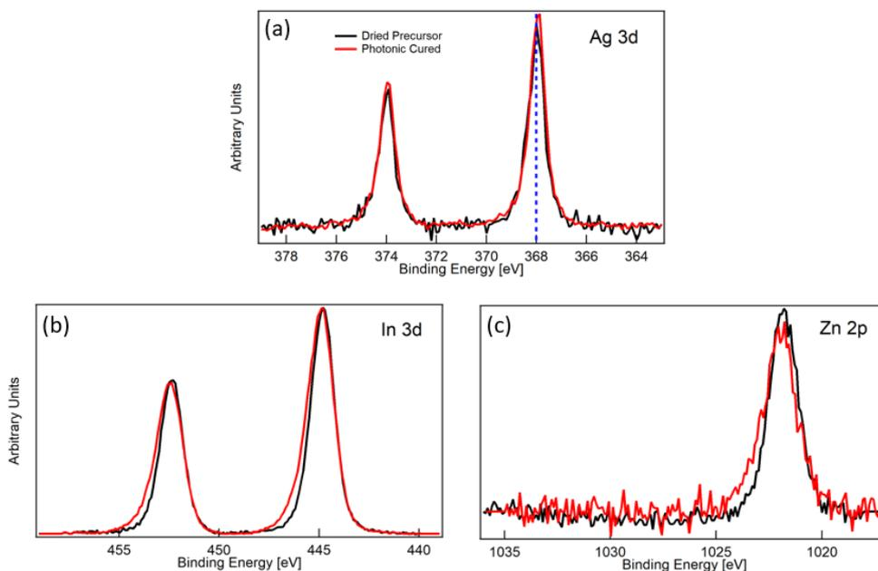
**Figure S5.** Normalized XPS spectra of precursor and final hybrid TCE: (a) Ag 3d, (b) In 3d, and (c) Zn 2p comparing the dried hybrid TCE precursor (black) and the final hybrid TCE after photonic curing (red).
