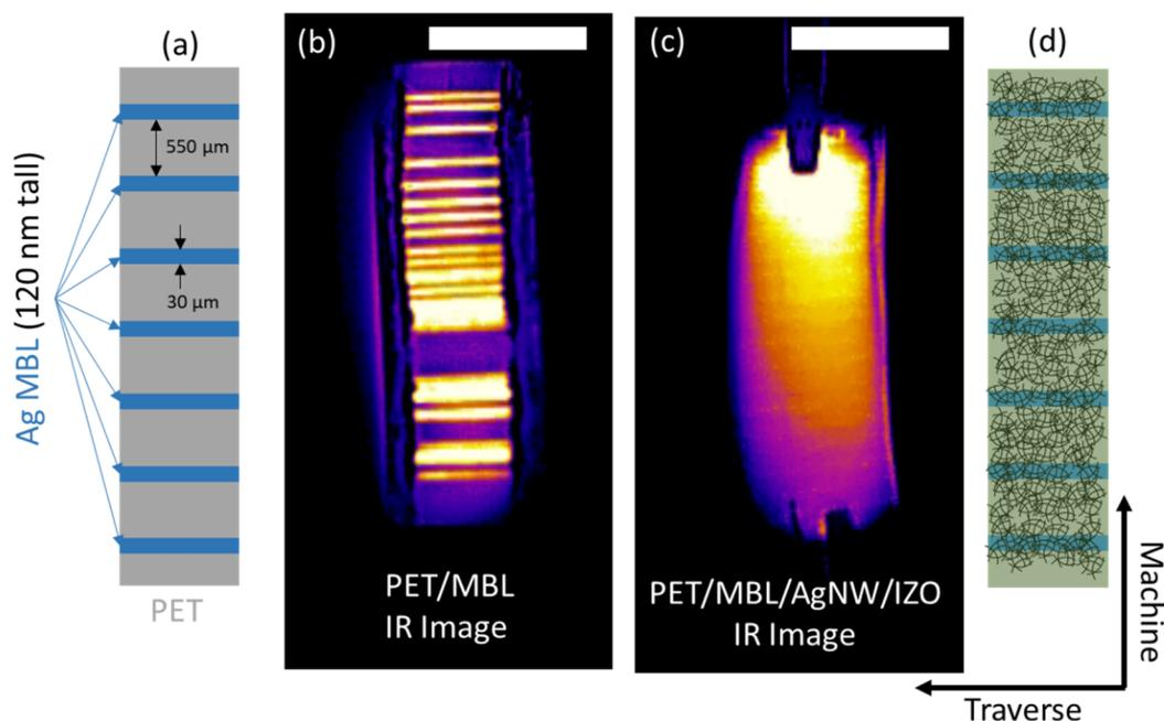
**Figure S9.** IR images of hybrid TCE: (a) PET/MBL substrate top-view schematic (PET in gray and Ag MBLs in blue), (b) IR image of a PET/MBL substrate under voltage bias applied to the long edges, (c) IR image of the hybrid TCE under voltage bias applied to the short edges, and (d) hybrid TCE top-view schematic (Ag MBLs in blue, AgNWs in black, and IZO in green). The voltage bias was  $\sim 2$  V. The scale bars in (b,c) represent 1 inch.
