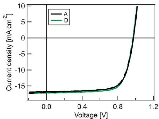
**Figure S16.** Champion PSC  $J$ - $V$  curves for stitching samples: Forward (dashed) and reverse (solid)  $J$ - $V$  scans for champion PSC made on hybrid TCEs placed at position A (black) and D (Green) during stitching photonic curing.
