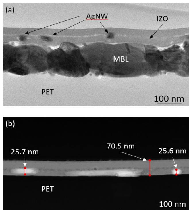
**Figure S7.** TEM and STEM cross section images of hybrid TCE: (a) TEM image of a hybrid TCE lamella taken from the MBL region, with PET, MBL, AgNWs, and IZO labeled. (b) STEM image of a hybrid TCE lamella taken away from the MBL. The AgNW diameters and total thickness of the two IZO coats are indicated. In both images the PET is at the bottom of the image.
