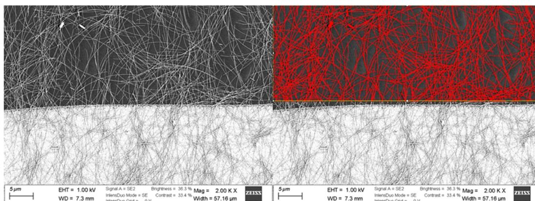
**Figure S10.** AgNW coverage: Representative SEM image of an AgNW-coated PET/MBL substrate at 2000x magnification before (left) and after (right) filtering the background using ImageJ. The analysis area selected was in the upper portion of the image (denoted by the thin yellow line and red colored AgNWs) to exclude the MBL feature. The red-colored AgNW area, as calculated from five different SEM images, was  $(28 \pm 5)\%$ .
