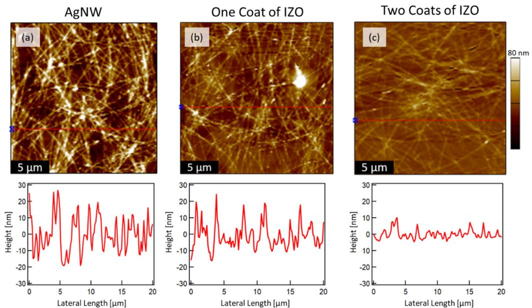
**Figure S4.** AFM images and height profiles of hybrid TCE: (a) after AgNW deposition, (b) after the first coat IZO, and (c) after the second coat of IZO on top of the PET/MBL substrates. The height profiles were taken along the red line shown in the AFM images.
