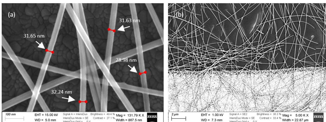
**Figure S1.** SEM micrographs of AgNWs: (a) High magnification SEM micrographs of Sigma-Aldrich AgNWs. The average diameter value from this image is  $31 \pm 1.5$  nm. (b) SEM micrographs of AgNWs near an MBL.
