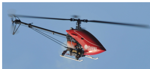
Figure 1. An unmanned helicopter that was independently developed by Stanford University. This photograph shows the Synergy N9 helicopter in flight, serving as the physical platform for experimental validation and the definition of the reference coordinate systems.
