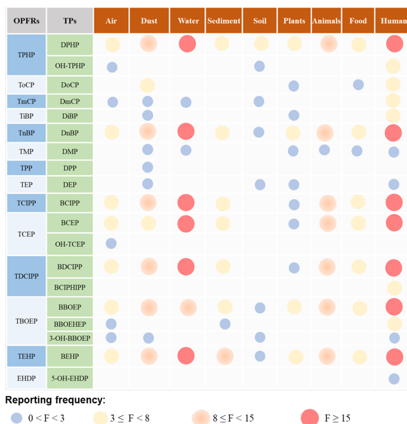
Figure 6. Detection of OPFR TPs in various environmental media. Abbreviations: DPHP: diphenyl phosphate; OH-TPHP: hydroxylated triphenyl phosphate; DoCP: di-o-cresyl phosphate; DmCP: di-m-cresyl phosphate; DiBP: diisobutyl phosphate; DnBP: di-n-butyl phosphate; DMP: dimethyl phosphate; DPP: dipropyl phosphate; DEP: diethyl phosphate; BCIPP: bis(1-chloro-2-propyl) phosphate; BCEP: bis(2-chloroethyl) phosphate; OH-TCEP: hydroxylated tris(2-chloroethyl) phosphate; BDCIPP: bis(1,3-dichloro-2-propyl) phosphate; BCIPHIPP: bis(1-chloro-2-propyl) 1-hydroxy-2-propyl phosphate; BBOEP: bis(2-butoxyethyl) phosphate; BBOEHEP: bis(2-butoxyethyl) 2-hydroxyethyl phosphate; 3-OH-BBOEP: 3-hydroxy-bis(2-butoxyethyl) phosphate; BEHP: bis(2-ethylhexyl) phosphate; 5-OH-EHP: 5-hydroxy-2-ethylhexyl diphenyl phosphate. The molecular structures of the above TPs are provided in Tables S7–S9 of the Supplementary Information.
