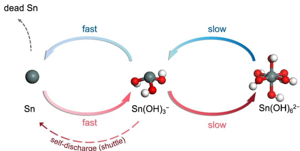
Figure 2. Schematic illustration of the four-electron transfer reaction at the aqueous tin anode.
