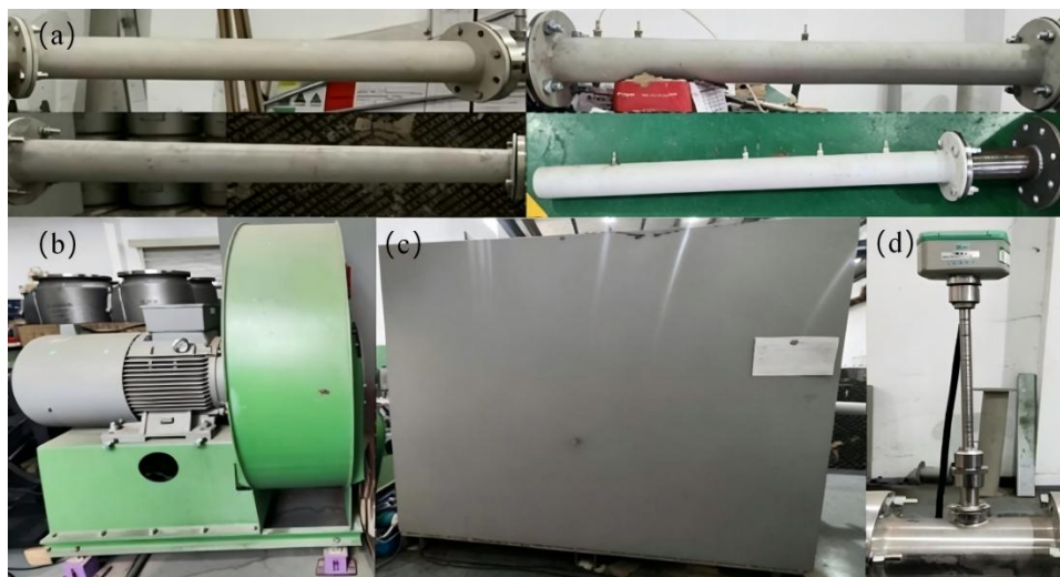
Figure 3. Experimental pipeline and fan system. ((a)-Test pipeline, (b)-Industrial fan, (c)-Gas storage chamber, (d)-Flow monitor).
