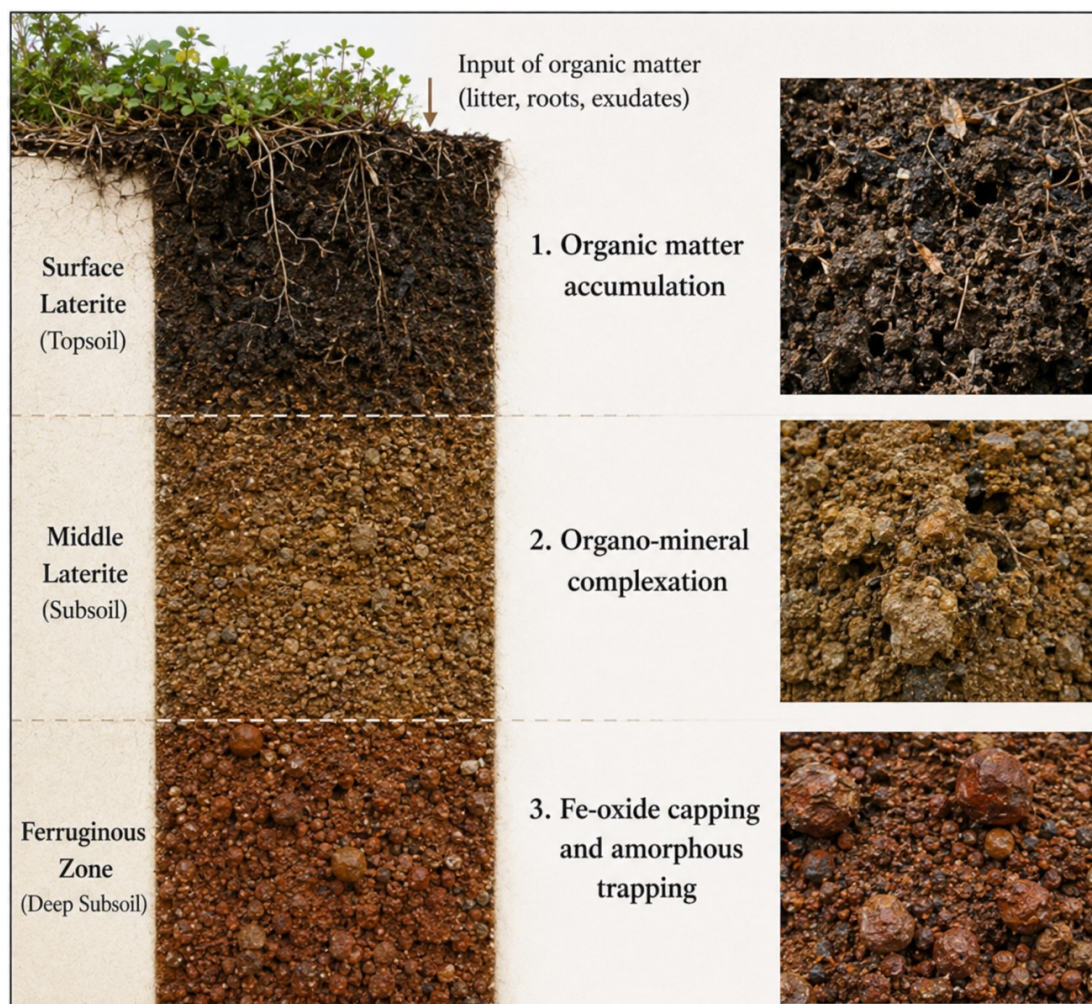
Figure 10. Schematic representation of carbon stabilization pathways in tropical laterites, showing organic matter accumulation, organo–mineral complexation, Fe-oxide-mediated protection, and long-term carbon preservation within lateritic horizons.
