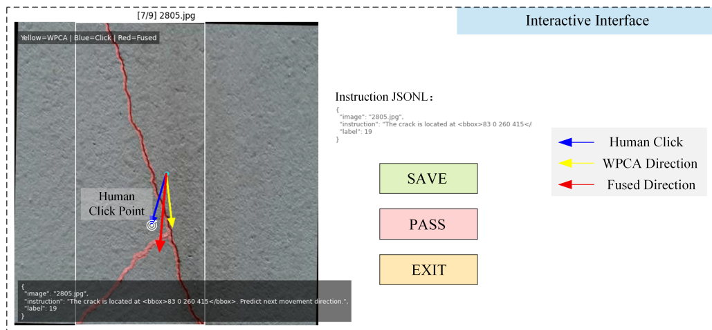
Figure 2. Human-in-the-loop direction supervision interface. The left panel supports click-based direction supervision, and the right panel previews JSONL records before export. The PASS button excludes from JSONL export any sample whose fused direction is ambiguous or unsuitable for supervision.
