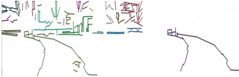
Figure 5. (Left): Curves extraction inspired by global precedence effect. Through grouping lines that follow proximity and continuity, a number of global whole curves are shaped, which has a higher visual priority to be perceived. (Right): Refined global curves. A number of global whole curves with higher parameters can be refined.
