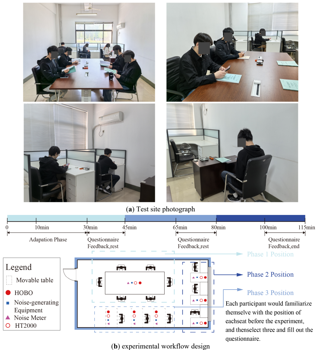
Figure 3. Site layout, equipment deployment, and three-stage operational workflow for the subjective experiment. (a) Test site photograph; (b) experimental workflow design.
