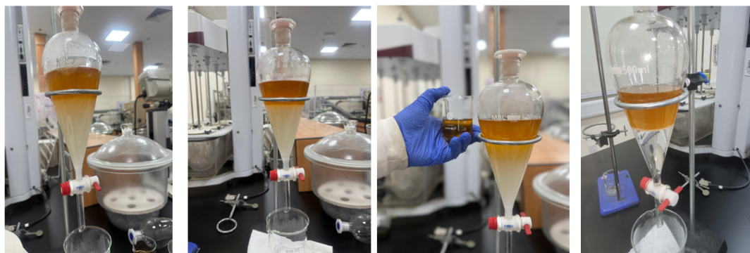
Figure 4. Schematic presentation of the three stages of the biodiesel washing cycle.
