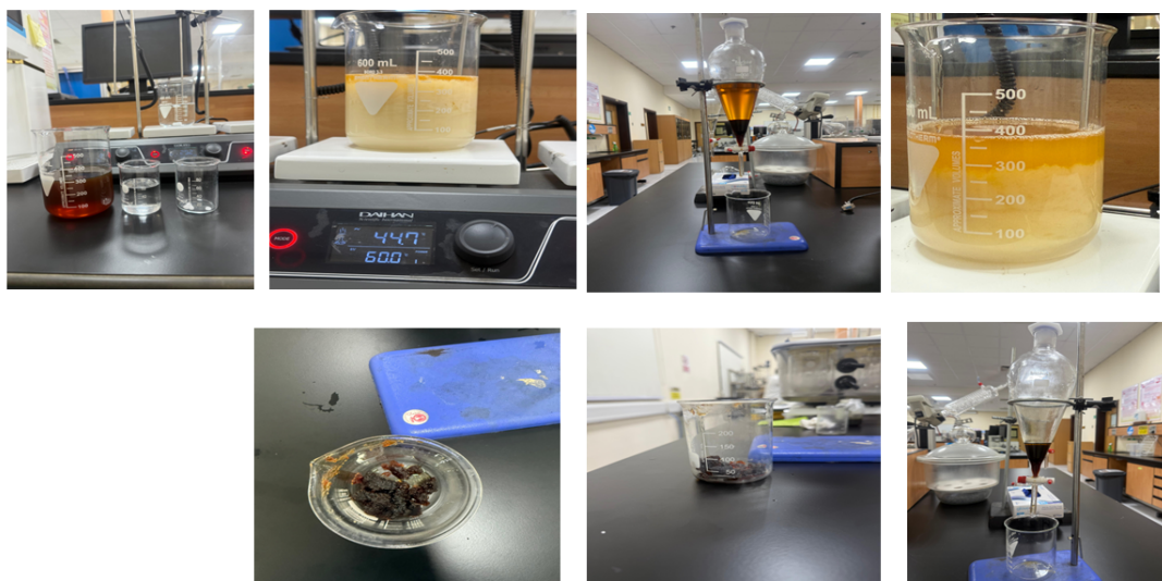
Figure 3. Steps of the biodiesel reaction and separation of glycerol.
