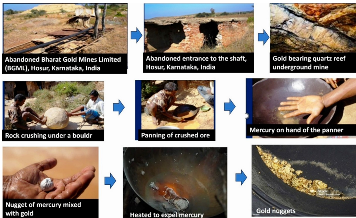
Figure 2. Different steps involved in the extraction of gold from gold ore using mercury, illegal gold mining practices in Hosur, Karnataka, India.
