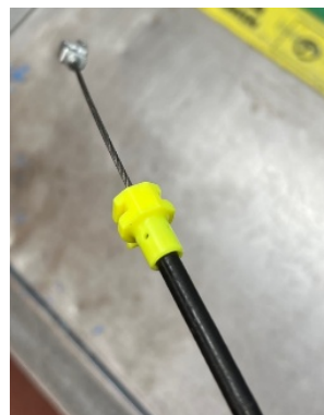
Figure 12. Correctly assembled end cable.
