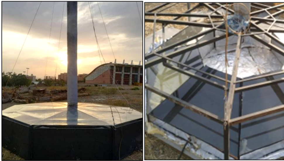
Figure 4. Solar Chimney setup in Iran University of Science & Technology, Tehran [29].
