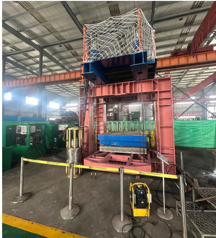
Figure 3. Scaled hydraulic synchronous lifting experimental platform.
