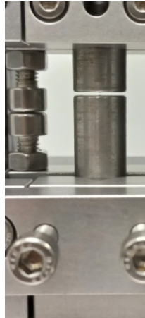
Figure 15. Substrate alignment and interfacial gap.
