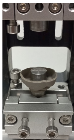
Figure 16. Silicone reservoir positioned on the lower substrate.
