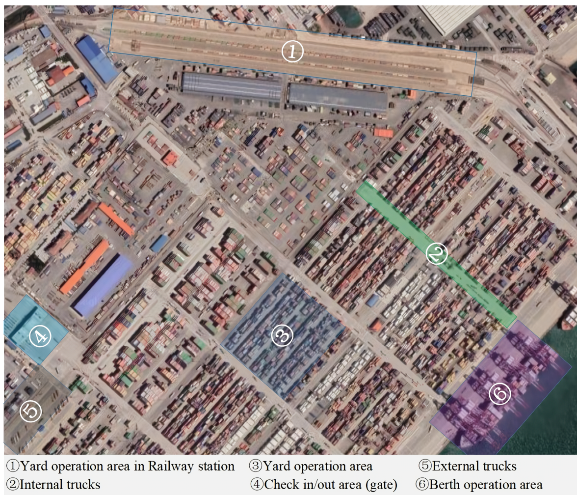
Figure 1. Layout of the container terminal and functional operation areas (Qingdao container terminal).
