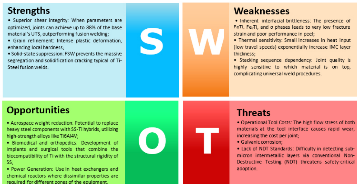
Figure 5. SWOT matrix for the dissimilar Friction Stir Welding (FSW) of Stainless Steel and Titanium alloys.
