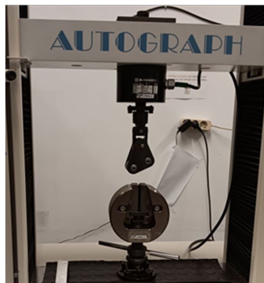
Figure 13. Shimadzu AG-I 10 kN tensile testing machine with a floating roller test apparatus installed.
