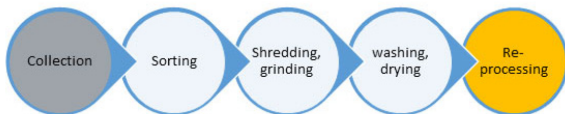
Figure 3. Circular economy model for additive manufacturing of recycled polymers printing (adapted from [129]).
