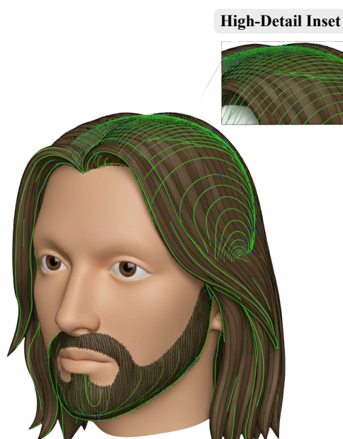
Figure 3. Toolpath planning over a 3D head model showing contour-parallel trajectories, tool orientation vectors, and a zoomed inset highlighting local path detail for controlled surface-following hair-cutting motion.
