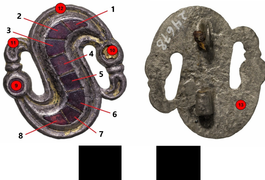
Figure 2. Front and rear side of ‘S’ shaped fibula—Sample n.: 24678 (from San Mauro hill, Cividale. Tomb n.:51). The numbers indicate the spots where the XRF (black on red background) and Raman (just black) spectra have been acquired. © Museo Archeologico Nazionale Cividale.
