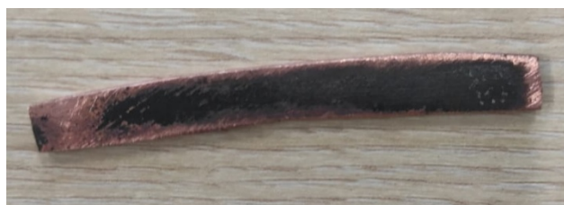
Figure 5. Metallic bar obtained after hot rolling of sintered Cu.
