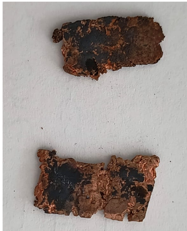
Figure 3. Metallic bars obtained after hot rolling of sintered CuproGraf powder.
