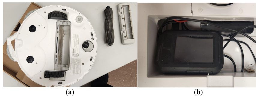
Figure 3. The mechanical integration of (a) the Dreame L10s Ultra smart vacuum, (b) an AccuRad detector and a Raspberry Pi.
