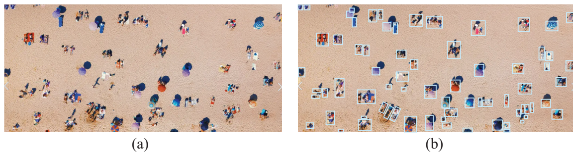
Figure 9. Illustration of the beach navigation scenario. (a) Original environment with static and dynamic obstacles. (b) Extracted obstacle boundaries for processing. The map dimensions are 50 m × 100 m, and all spatial measurements are in meters (m).
