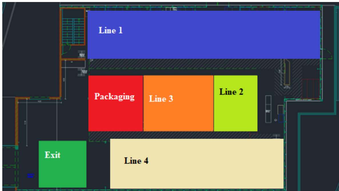
Figure 2. Assembly Line Layout. • Line 1 (Trolleys, Monoblocs and Stretchers); • Line 2 (Chairs); • Line 3 (Tables, Ramps and Stirrups); • Line 4 (Platforms and Carts).
