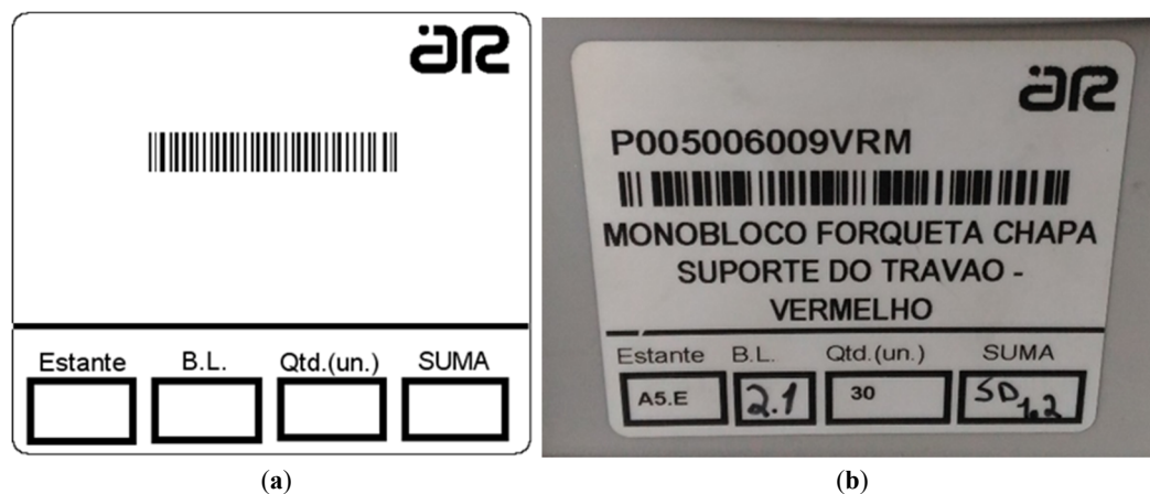
Figure 4. Kanban Card (a) and Kanban Card Application Example (b).
