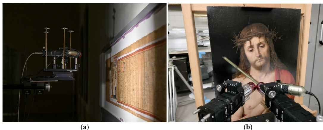
Figure 1. Portable micro SORS set-up implemented during the MOLAB analytical campaign at the Museo Egizio (a) and Museo Poldi Pezzoli (b).
