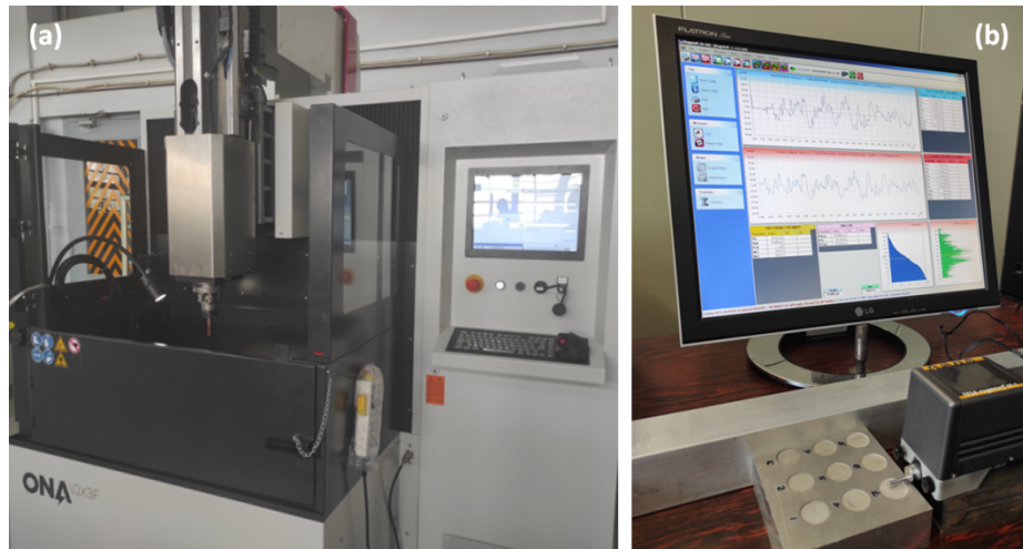
Figure 1. EDM experimental setup and roughness measurements: (a) EDM machining setup; (b) Roughness measurements and corresponding measurement processing environment.
