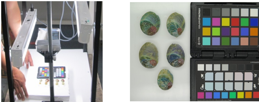
Figure 1. The light table and digital camera ( left ) were used to capture images of greenlip abalone ( H. laevisgata ), and a reference colour card ( right ) was used to convert the pixels to length in mm.
