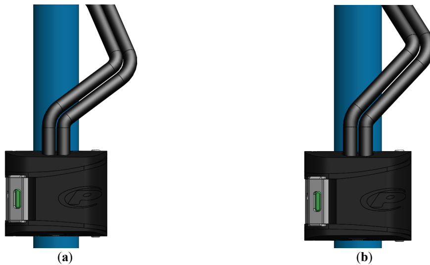
Figure 14. Connection rod curvature relaxation, (a) before the relaxation procedure, (b) after the relaxation is completed.
