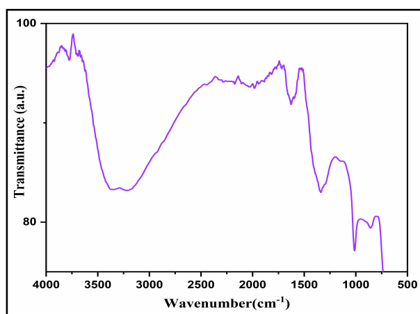
Fig. 4. Representation of FTIR of synthesized iron oxide nanoparticles.
