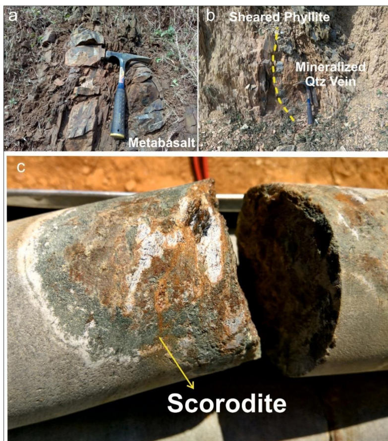
Figure 3. (a,b) Field exposures showing sheared metabasalt and mineralized quartz veins localized along the S_1 and S_2 foliation planes within phyllites; (c) Drill core sample illustrating the alteration of arsenopyrite into porous, light bluish-green scorodite within phyllitic host rock.
