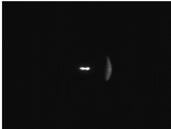
Figure 12. Peripheral PSF at 45 degrees using an iris of 3 mm and a distance between the IOL and the iris of 1.5 mm.
