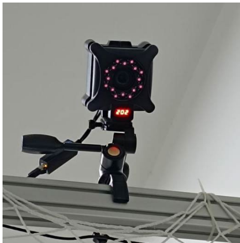
(b) NOKOV high-speed infrared motion capture camera
