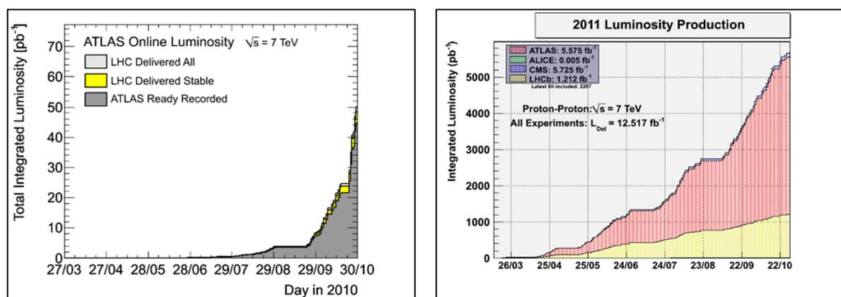
**Figure 10.** Plots show the daily progress in performance of the LHC in 2010 and 2011, reaching a maximum of 44 in 2010 and 6000 in 2011.
