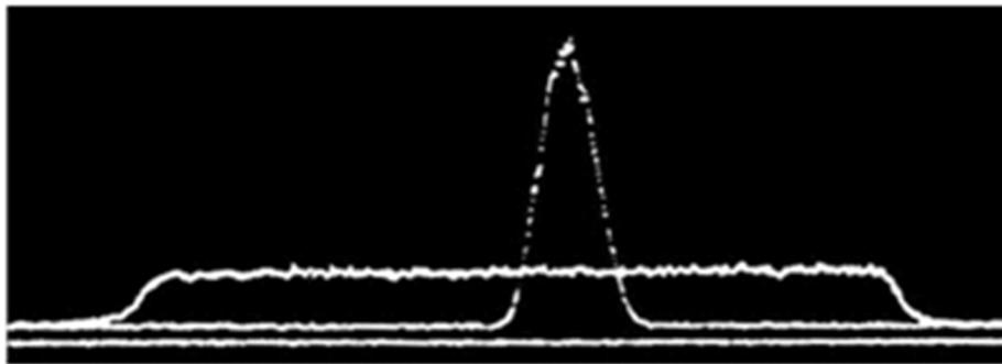
**Figure 5.** Fast momentum cooling in ICE.
