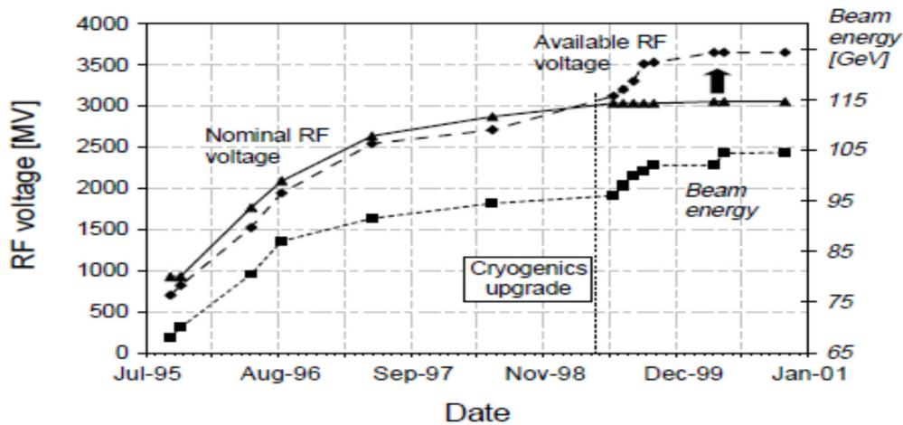
Figure 7. RF voltage per turn over the years.
