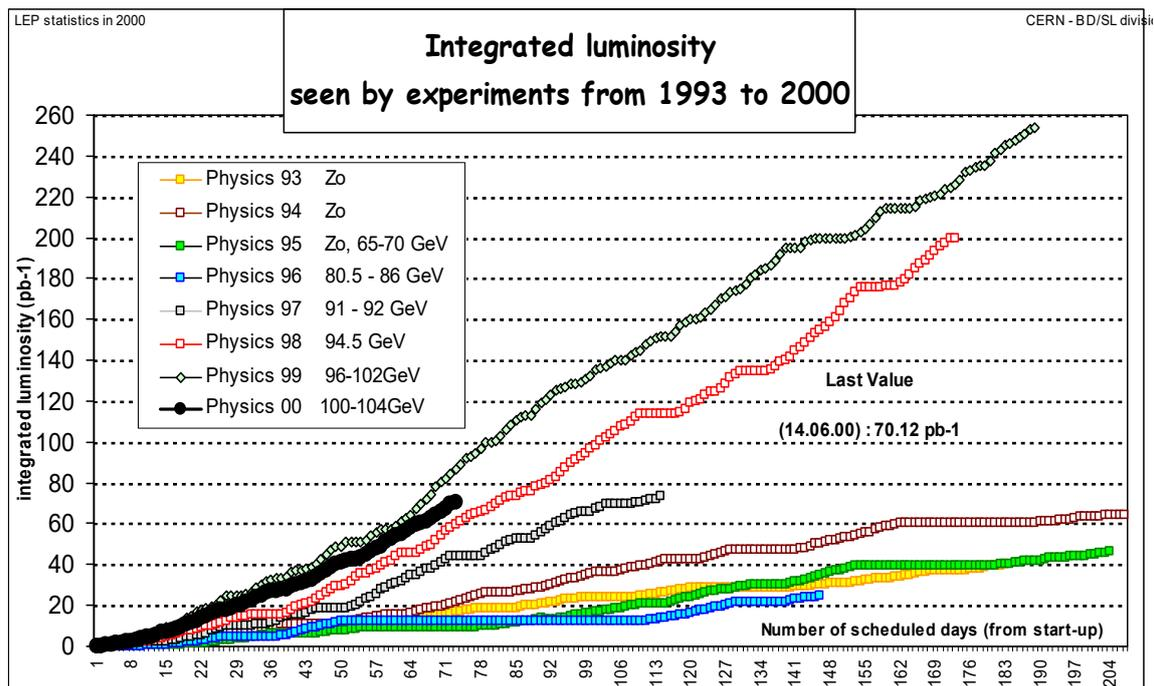
Figure 8. LEP daily integrated luminosity from 1993 to 2000.
