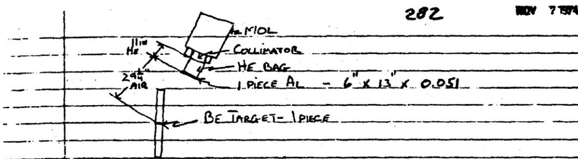
**Figure 21.** Aluminum foil arrangement in front of magnet  $M_0$  in our new experiment to determine the  $e/\pi$  ratio. The converter was used to determine the electron background yield.
