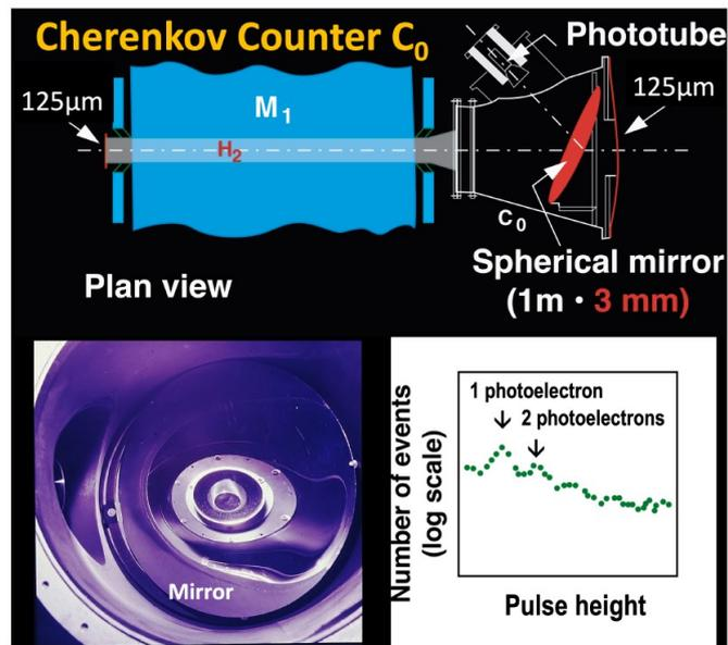
**Figure 18.** The  $\pi - e$  separation was achieved by four extremely sensitive Cherenkov Counters  $C_o$ ,  $C_e$ .
