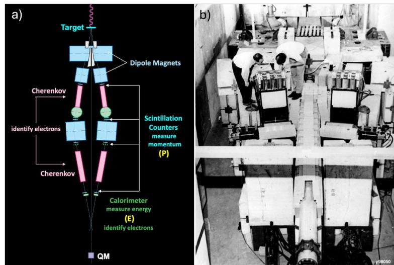
**Figure 2.** (a) Experimental layout of my experiment for electron size measurement at DESY; (b) Photo of the experiment for electron size measurement.
