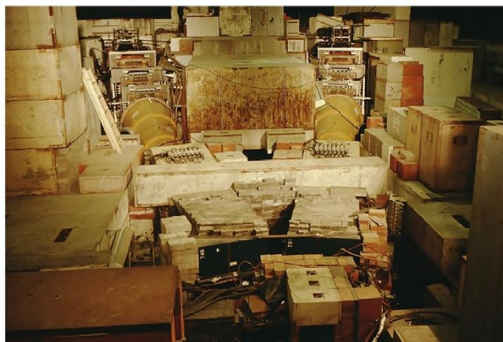
**Figure 13.** Shielding arrangement with roof open.
