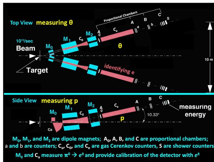
**Figure 12.** Layout of the AGS Experiment E598, which is an upgraded precision version of the DESY experiment.
