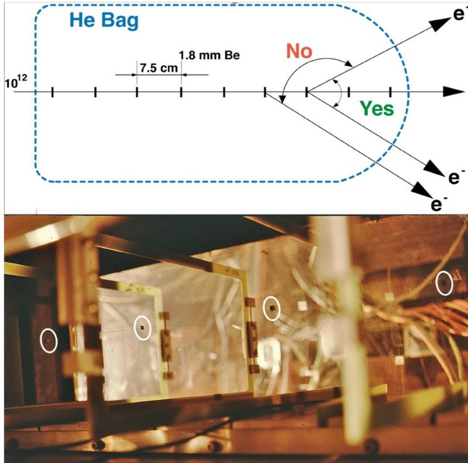
**Figure 14.** Nine separate targets to reduce the background.
