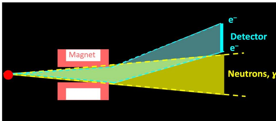
**Figure 15.** The magnets bend charged particles to an angle such that the detectors are not exposed to photons or neutrons from the target.
