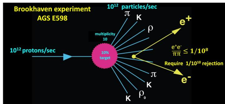
**Figure 11.** Concept of the AGS Experiment E598. The extracted beam of  $10^{12}$  protons/s interact with a 10% target. The multiplicity is 10, resulting in  $10^{12}$  particles/s from the target volume. The ratio  $e^+e^-/\pi^+\pi^-$  is less than  $1/10^8$ , so a percent accuracy measurement requires  $1/10^{10}$  rejection.
