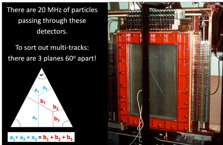
**Figure 17.** Precision position detectors, which were designed by the late Professor UJ Becker. The chamber, shown on the right, is on display in Smithsonian Institution in Washington, DC after completion of the experiment.
