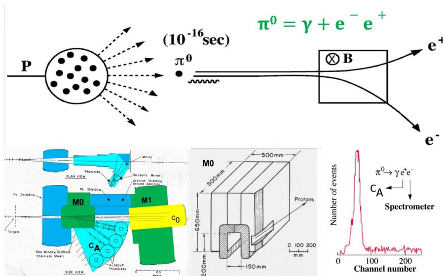
**Figure 16.** Detector calibration with a pure electron beam by placing a specially designed magnet  $M_0$  close to the target followed by a special Cherenkov counter,  $C_A$ , to detect positrons from  $\pi^0 \rightarrow \gamma e^+ e^-$  ensuring the electron entering the spectrometer.
