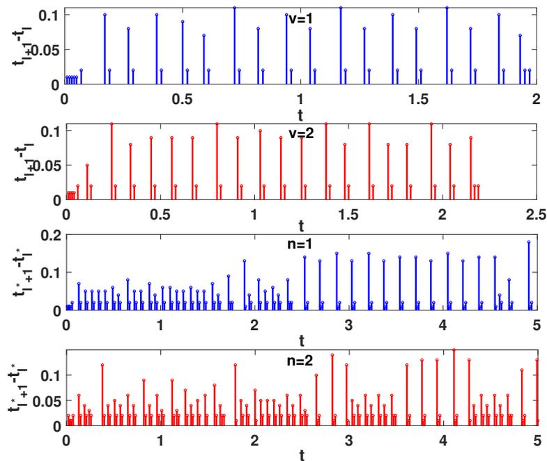
**Figure 10.** The time transmission intervals of ETC (43) and (44).
