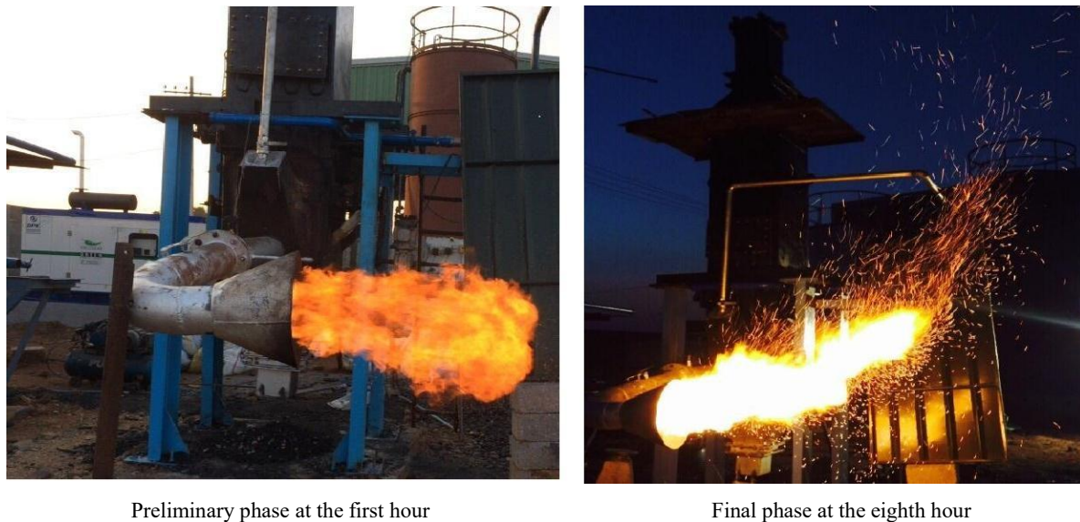
Figure 3. Producer gas flame from MSW gasification utilized at various operational stages.
