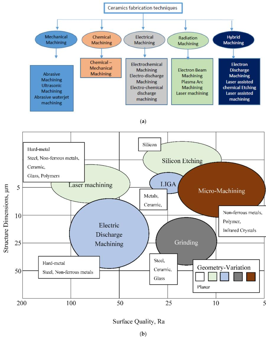
Figure 5. (a) Ceramic fabrication techniques, (b) EDM and micro-EDM relatively to other manufacturing processes on CMC [77].
