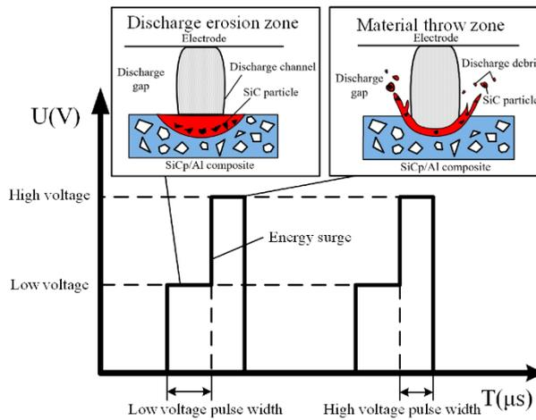
Figure 4. High- and low-voltage composite waveform [76].
