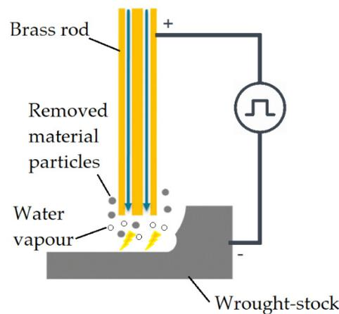
**Figure 1.** Schematic of the EDM discharge process and material removal [10].
