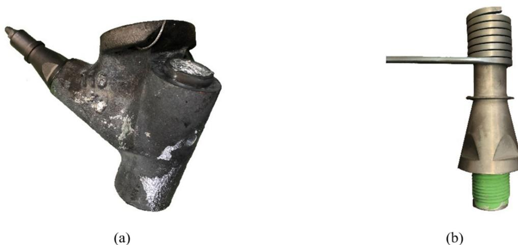
**Figure 1.** (a) Injection nozzle assembled in the hot-chamber die-casting machine, and (b) nozzle with the electrical resistance assembled on its tip.
