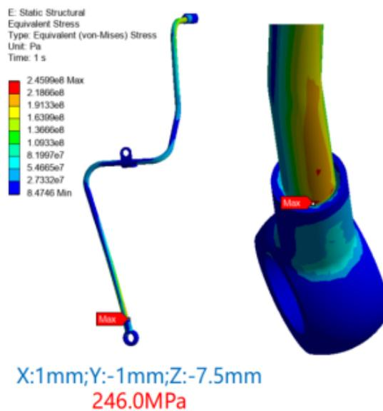
**Figure 15.** Simulation stress of sample 5#.
