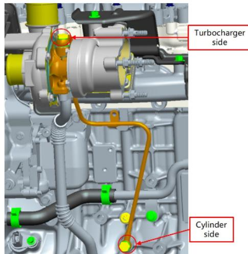
**Figure 11.** Pre-tighten bolts at both ends.
