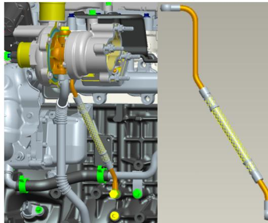
**Figure 16.** Preparation of the hose structure booster inlet pipe.
