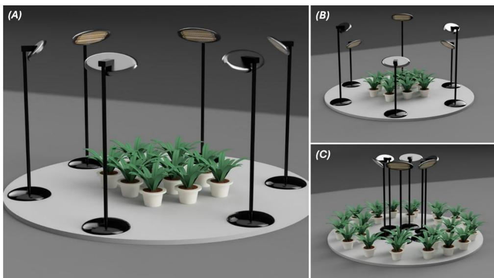
**Figure 2.** Basic configurations examined to study the combination of parameters that resulted in better thermal homogeneity. Configuration 2A shows a plot of plants surrounded by 6 heaters located at the same height over the vertices of a hexagon. Configuration 2B shows the same plot surrounded by 6 heaters placed at staggered different heights over the same vertices. Configuration 2C shows the heaters in the centre, surrounded by plants forming a circle.
